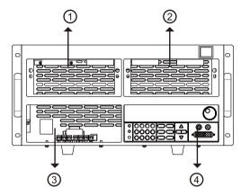
1,2,3 and 4 can be used for connecting OVP power, AC/DC power, electronic load, switch analyzer, etc.
